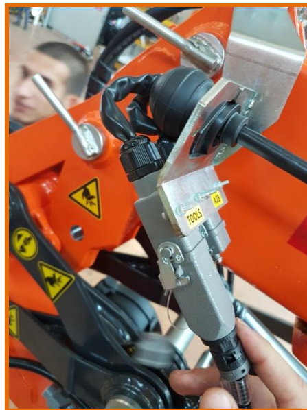
“TOOL” plug on tip of the main boom
